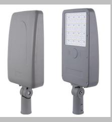
AIRRO solar led street light is dedicated to provide continuous and ultra high brightness output for main road market. It build in big capacity of LifePO4 battery pack up to 768WH max whose lifetime could reach to more than 10 years in energy saving mode, and It equips 64pcs of SMD5050 (5W/led) as lighting engine, it is derived by constant voltage and lower current in order to get superb high luminous output up to 180lm/W.
